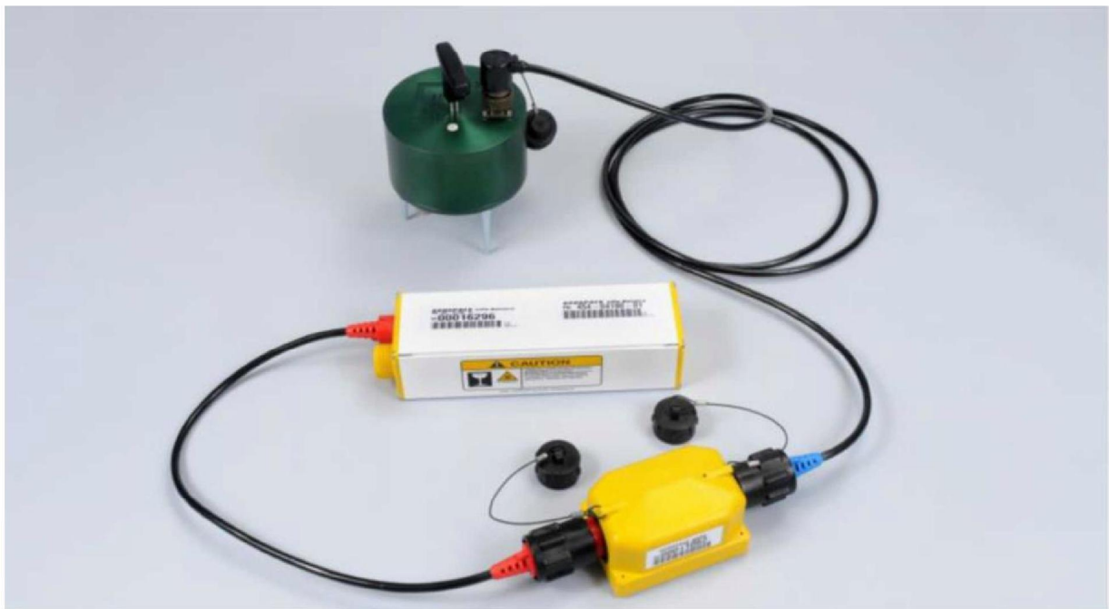
Figure 3.2 Node of the flexible geophone network consisting of the battery pack (white), data logger (yellow) and three component geophone (green).
