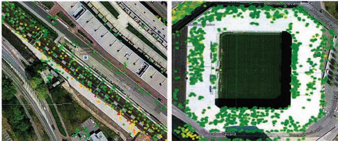
Fig. 4.6 InSAR measurements; Left: from ground (< 3 m in height). Right from top of buildings (> 3m)
