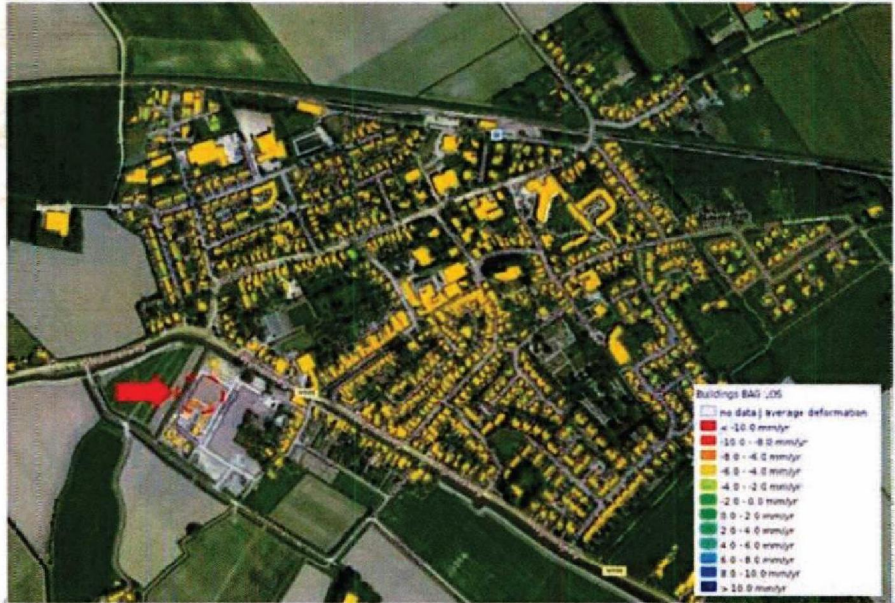
Fig. 4.4 Subsidence rate per building derived from InSAR measurements. A faster subsidence (highlighted in the dashed circle) than its neighbours suggests the building may have foundation or structural issues.
