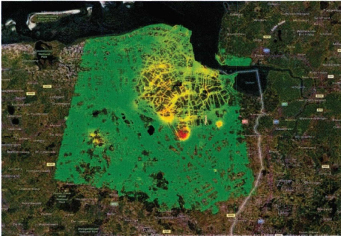
Fig. 4.3 InSAR (TSX 3 m resolution) measurements over Groningen.
