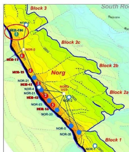
Figure 1.4 – Geological map of the NOR Field, including leaning well NOR-416 (green) and the Norg expansion wells (red)
